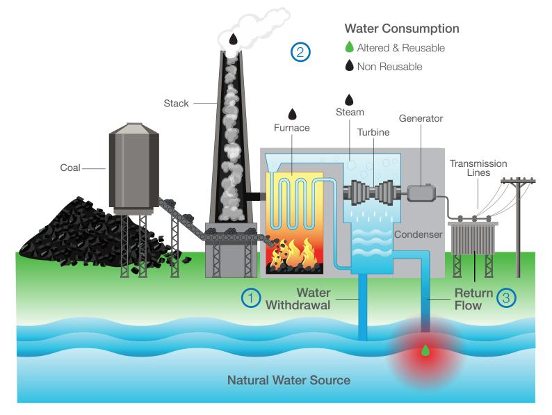
Water is withdrawn from a natural water source and pumped into the coal plant.
